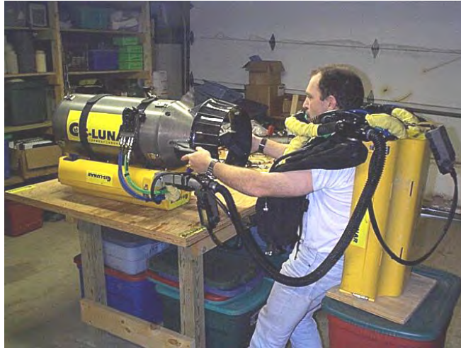
Figure 5. Stone and his group developed a bailout system mounted onto a diver propulsion vehicle (DPV) for the Wakulla 2 project, but it was not popular with the exploration divers. Photo courtesy US Deep Caving Team, Inc.
